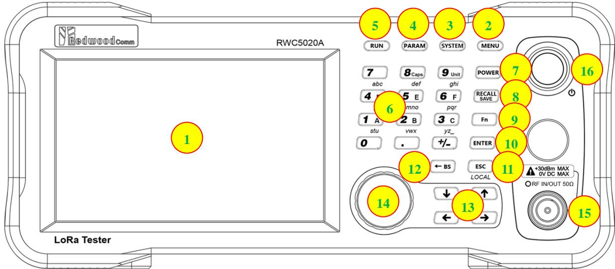
Fig 2.1 RWC5020A/B Front Panel View
