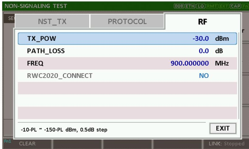
Fig 3.32 RF Parameters for Signal Generator
