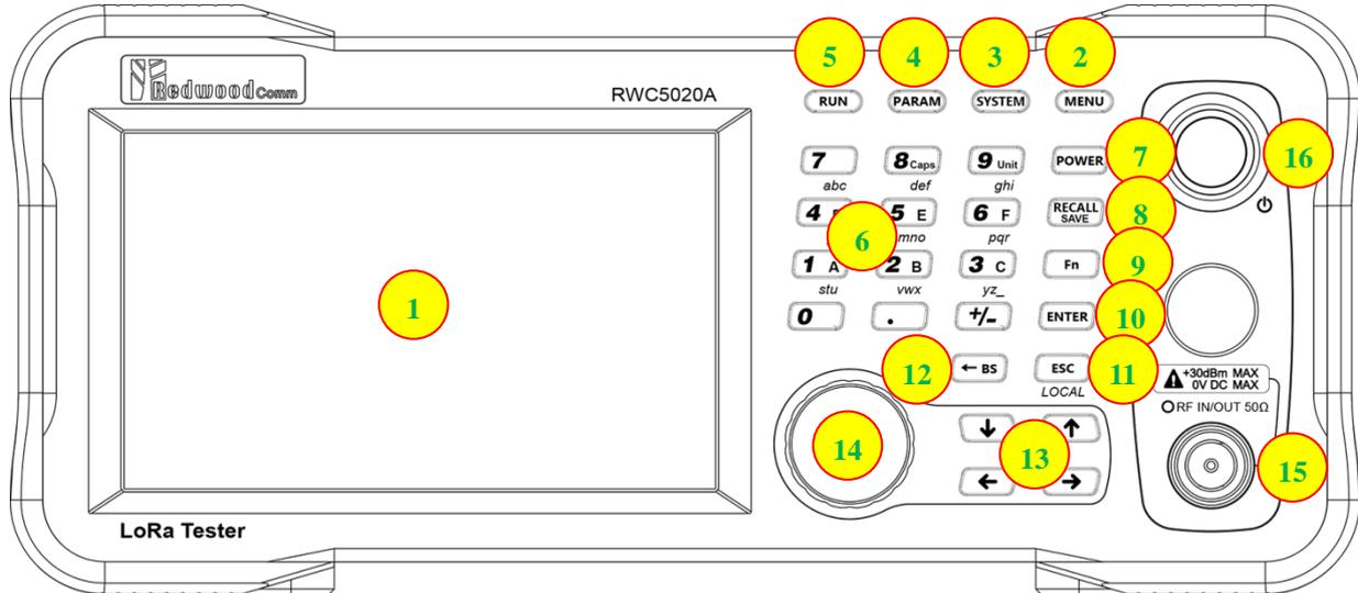
Fig 2.1 RWC5020A/B Front Panel View
