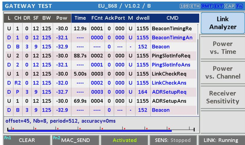
Fig 3.30 Example of communication with Class B Gateway
