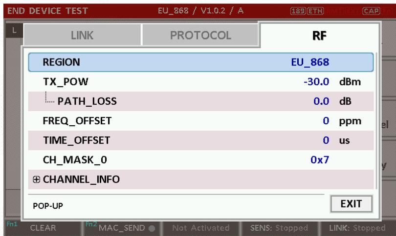
Fig 3.2 EDT Parameter Configuration Screen - RF
