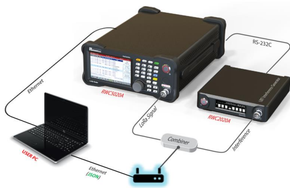
Fig 3.29 CW Interferer test environment
