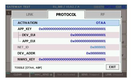
Fig 3.21 Parameters for OTAA (LoRaWAN V1.0)
