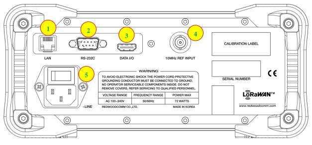
Fig 2.2 RWC5020A/B Rear Panel View
