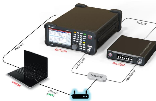
Fig 3.27 CW Interferer test environment
