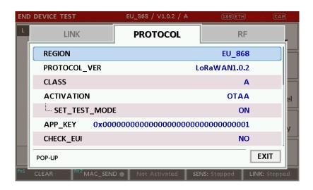
Fig 2.5 Parameter Configuration Screen
