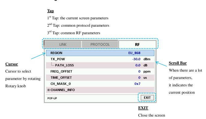
Fig 2.9 Parameter Configuration Screen
