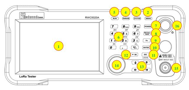
Fig 2.1 RWC5020A Front Panel View
