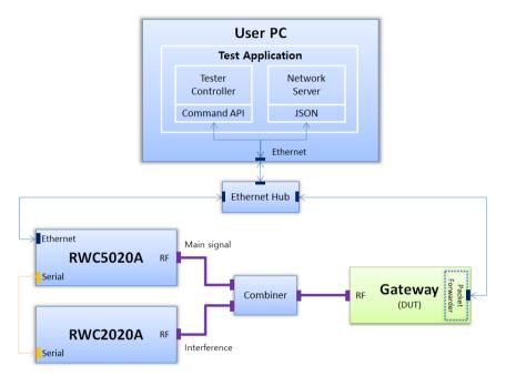
Fig 1. Conceptual Block Diagram
