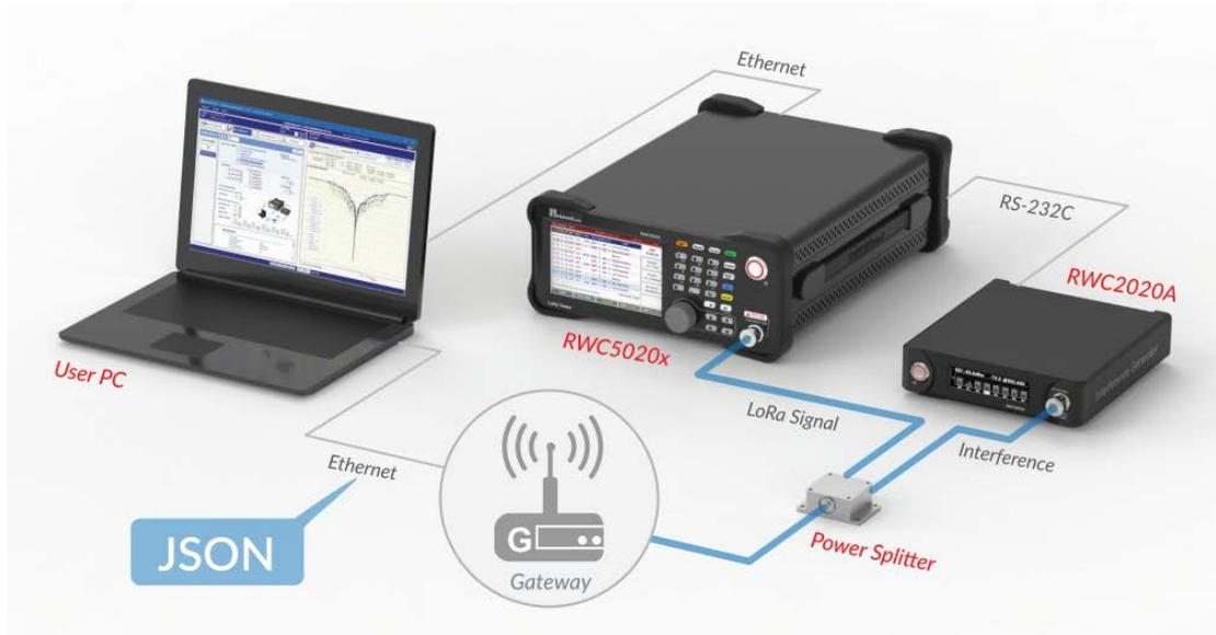
Fig 3. Gateway Test Setup
