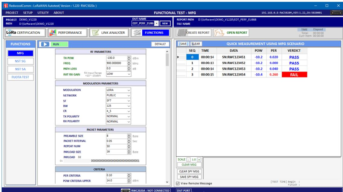
Fig 3.47 Example test using 4 DUTs(N=50, Target PER=0.1)
