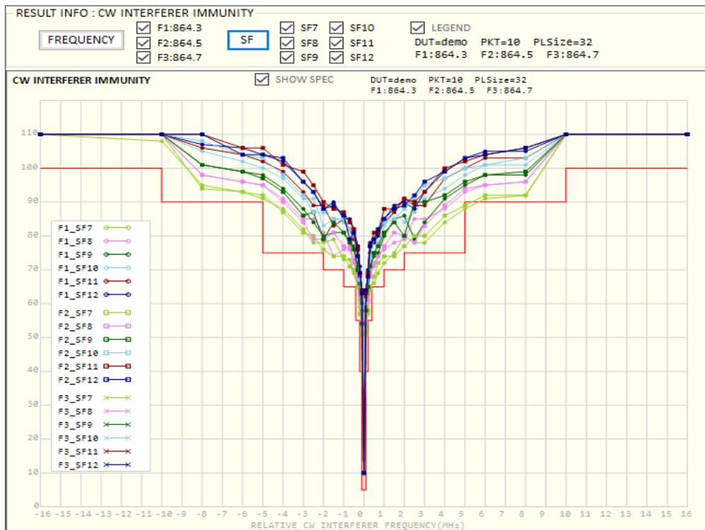
Fig 3.31 The test result of CW Interferer Immunity
