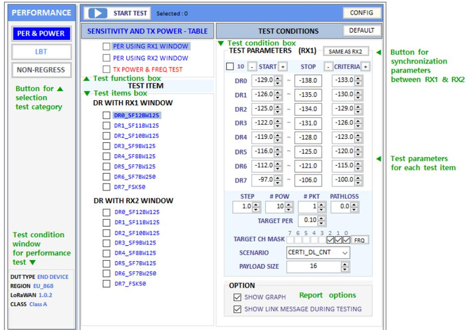
Fig 3.10 Test parameters and conditions
