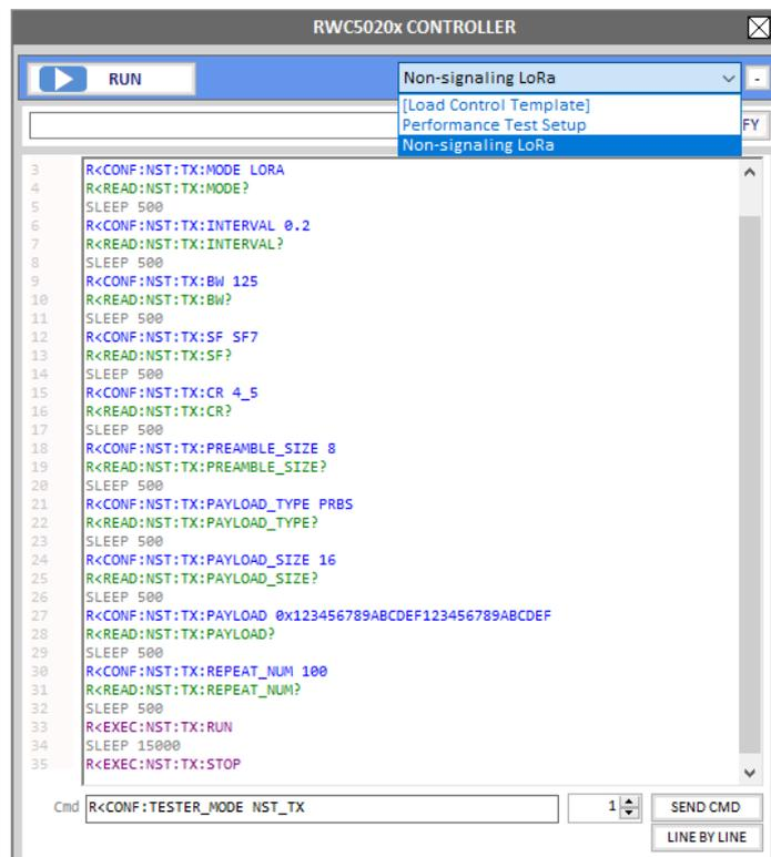
Fig 3.57 Sending commands of RWC5020x Control window
