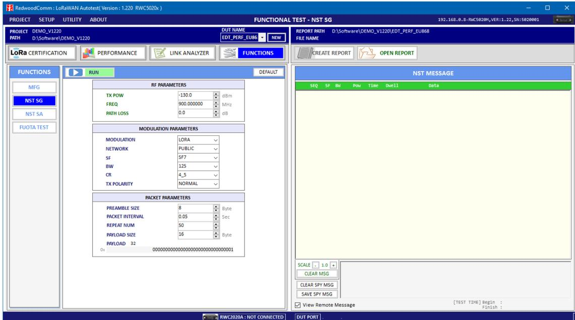
Fig 3.48 NST SG parameters and report window
