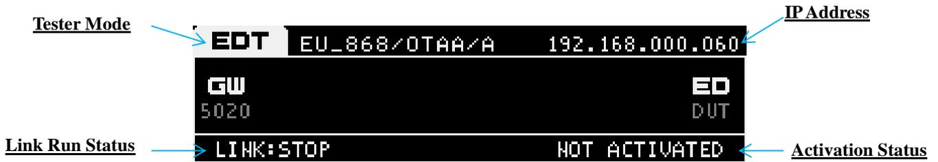
Fig A.3 RWC5020M Screen in IDLE state
