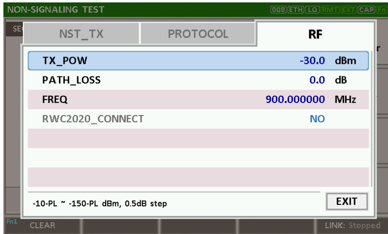
Fig 3.32 RF Parameters for Signal Generator
