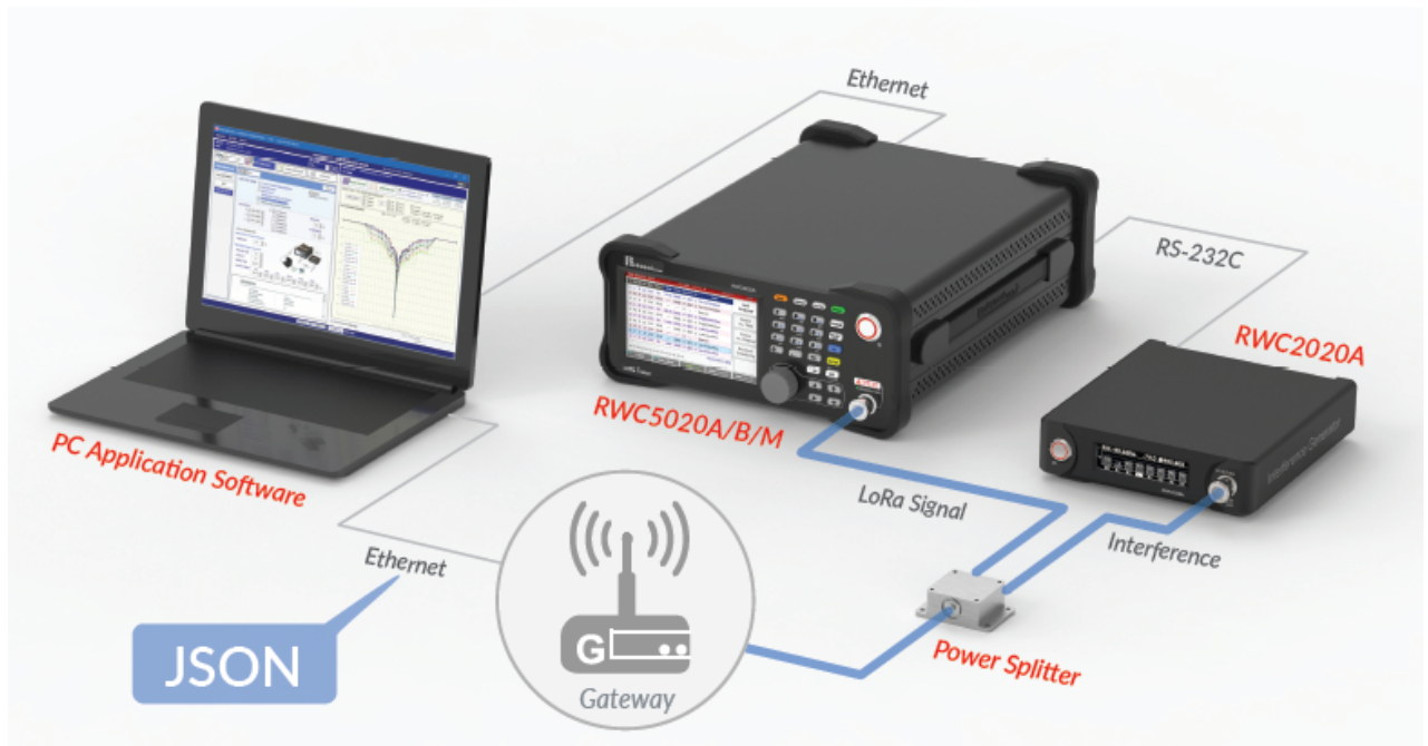
Fig 3.25 The Concept of non-regression test of gateways
