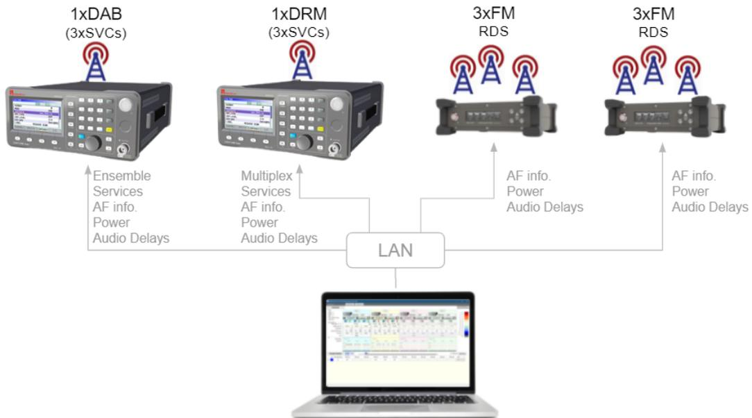
Figure 1.3 Service Linking test environment using RWC2010Bs and RWC2100Fs
