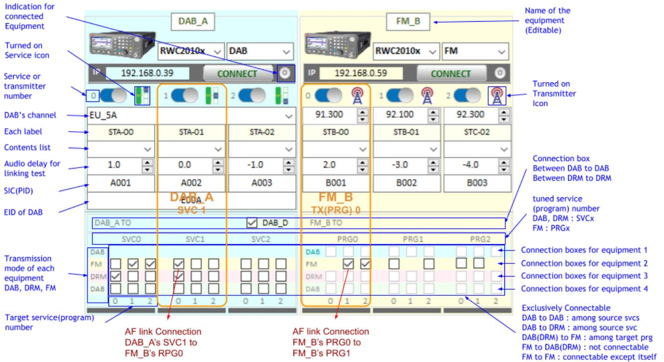
Figure 1.5 Indications and parameters for stations
